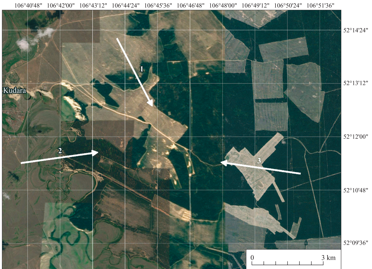
Fig. 3. Test area on the Google Maps and geometry of radar imaging for SIR-C (arrow 1) and ALOS PALSAR at ascending (arrow 2) and descending (arrow 3) orbits.
